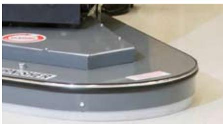
Polivac's 'floating skirt' and Total Dust Control Vacuum System traps all polishing dust for a beautiful finish.
