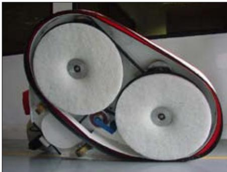
Counter-rotating 'Jackaroo' pads, combined with the 'flexible' pad holder and pulley system means both pads constantly follow the contours of the floor – giving an exceptionally smooth and even finish.
