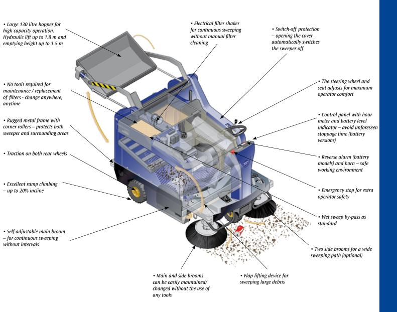
The FLOORTEC R680 series includes a battery (B) and a petrol (P) model, both available with 800 mm main broom and one side broom (1050 mm sweeping path). In case you want to add on extra equipment to match specific cleaning needs we provide a wide selection of options to choose from.
