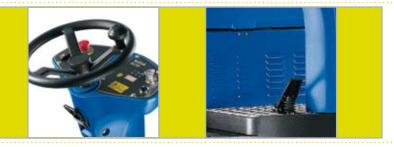
Adjustable ergonomic steering column to suit all operators. Ergonomic foot pedal with forward/reverse switch on control panel
