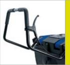
Adjustable ergonomic drive handle to match operator height. Foldable for easy transport.
